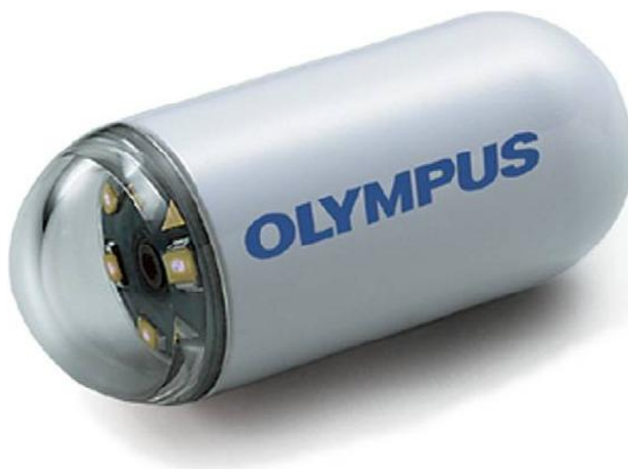
Fig. (1) Endocapsule (Olympus) for the small bowel is 26 x 11 mm, weighs 3.8 g, has a field of view of 145 degrees, uses 6 white LEDs, and has a battery life of 8 hours.
