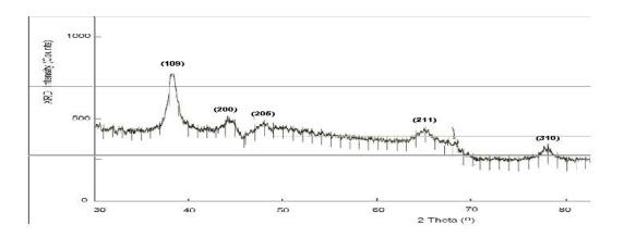
Figure. 3 XRD spectra of silver nanoparticles synthesized using 2 g wet biomass of *Mangifera indica* incubated with 1 mM AgNO<sub>3</sub> for 3 days.
