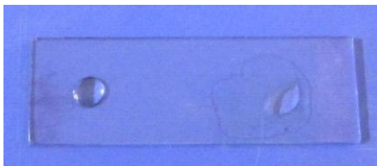
Fig .4 Drop collapse method
