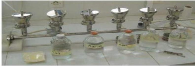
Figure 2 : Membrane filtration technique
