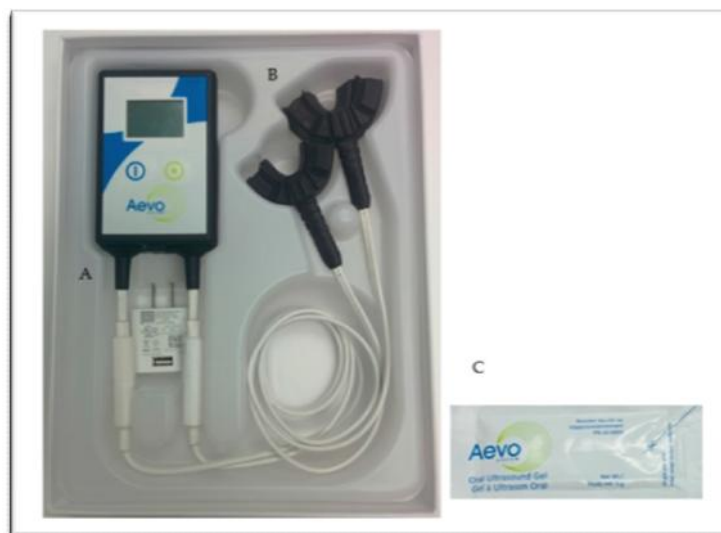
Fig 22: Low-intensity pulsed ultrasound (LIPUS) device (Aevo System). (A): Handheld electronics; (B): mouthpieces; and (C): ultrasound coupling gel.
