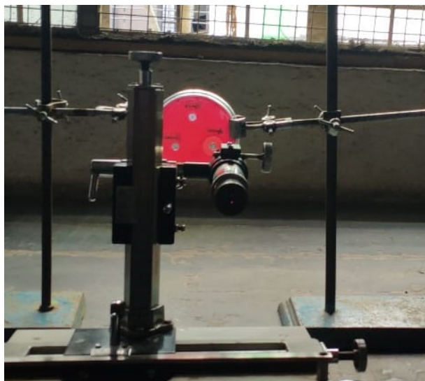
Figure 2: Measurement of diameter of inhibition zone by travelling microscope
