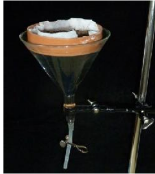
Figure 11 Baermann funnel method Sample extraction
