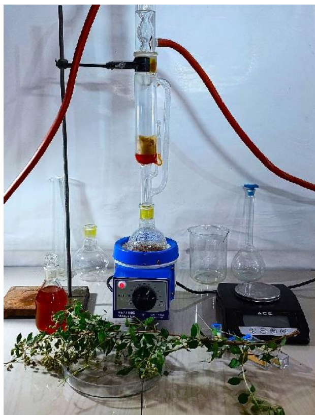
Fig.-3 Showing Lawsonia inermis extraction by using Soxhlet apparatus
