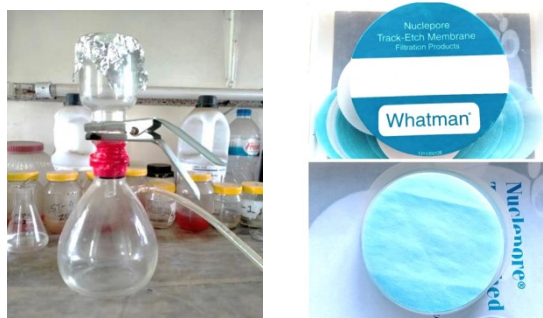
Figure 3: Microplastic items filtration process
