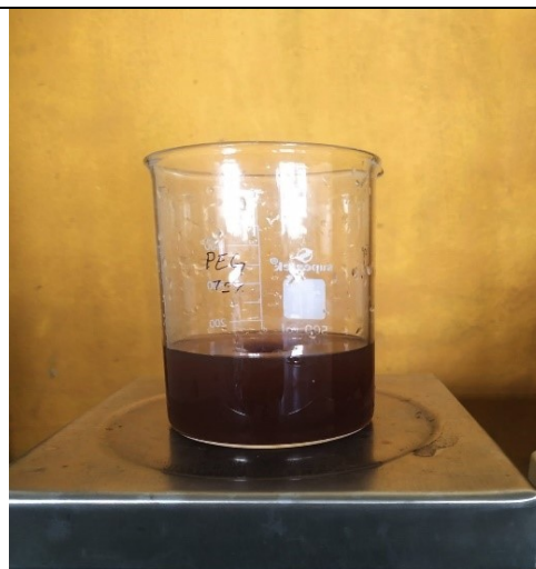
Figure 2. Constant stirring of TTIP solution with the extract of Azadirachta indica in 1:1 ratio (v/v basis)
