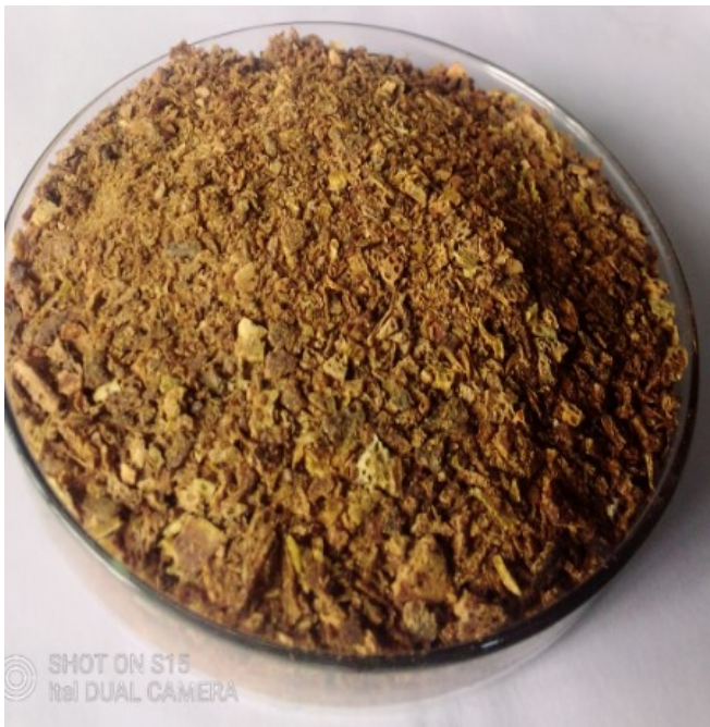
Plate 2: The plate showing grinded and dried orange peels. Adsorption process on Orange Peels
