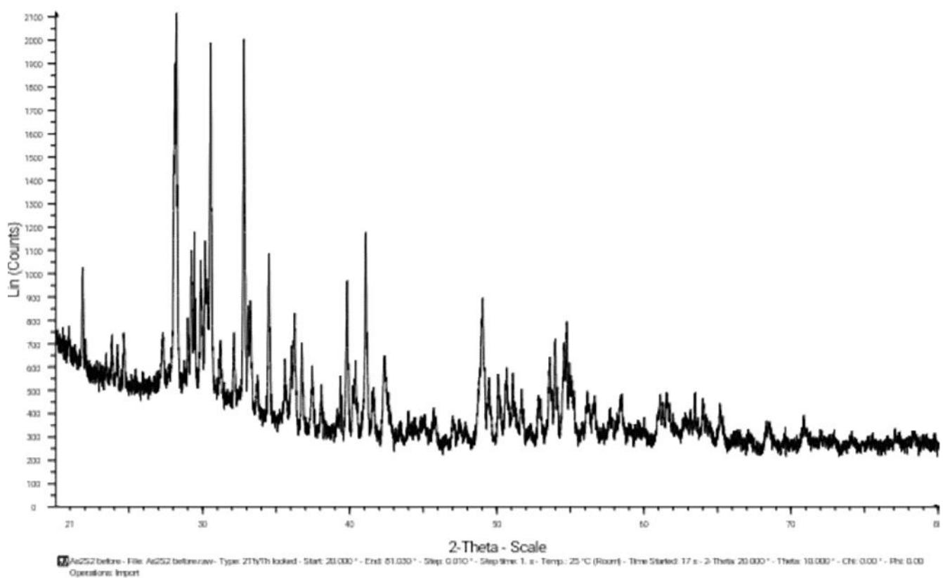
**Figure 5: XRD pattern of Test Sample AsS before Purification**
