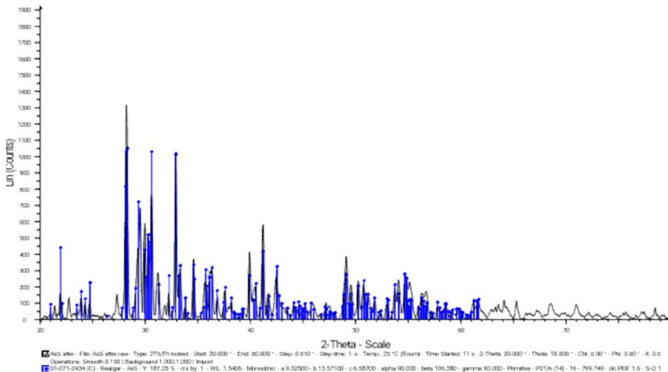
Figure 6: XRD pattern of Test Sample AsS after Purification
