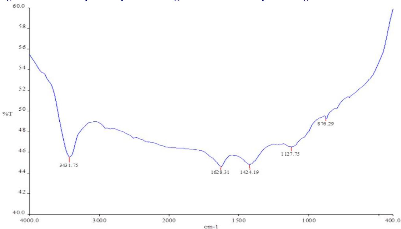
The FT-IR absorption spectrum of the sample Mansolai after purification reveals that the IR absorption peak at 1420.18 cm<sup>-1</sup> due to presence of S=O functional group stretching. Vibrational peak at 3409.68 cm<sup>-1</sup> maybe due to the presence of primary
