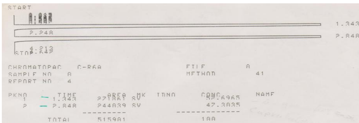
Figure (4-a): HPLC of the standards: 6- amino hexanoic acid with retention time 1.343 and caprolactam with retention time 2.848
